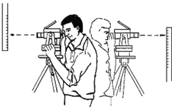
Figure 4.1 Using a dumpy or surveyor's level and staff to measure head (courtesy of BHA)
