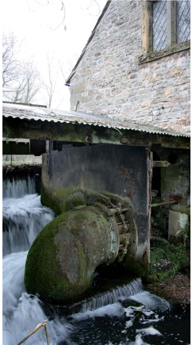
Figure 2.12 An original Francis turbine in situ at Flewitt's Mill, Ashford in the Water
